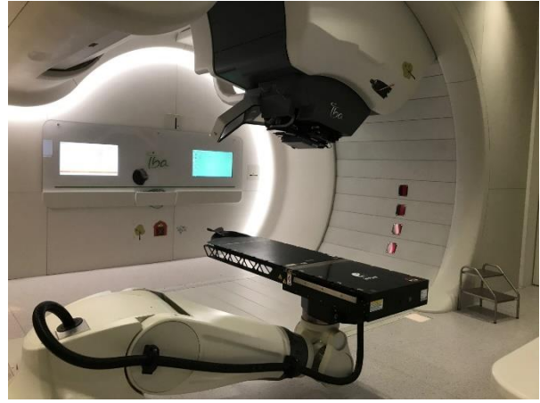
The Centre François Baclesse uses Proteus One proton therapy equipment (by IBA) which has a mobile gantry system with pencil-beam scanning (PBS), allowing conformational treatment with 3D modulation of the dose delivered.
